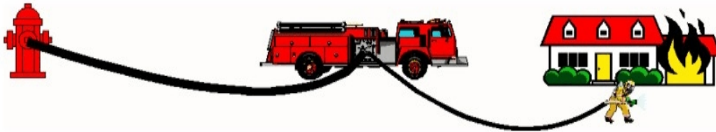
Figure 6 - Example of a Forward Lay
